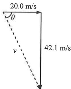
$$\begin{aligned} v_R &= \sqrt{v_x^2 + v_y^2} \\ &= \sqrt{(20.0 \text{ m/s})^2 + (41.2 \text{ m/s})^2} \\ &= 45.8 \text{ m/s} \end{aligned}$$
